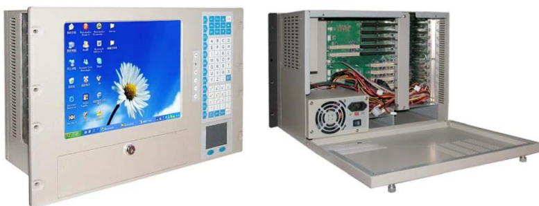
19" 7U 10 Slots 12.1" TFT LCD Workstation Chassis
